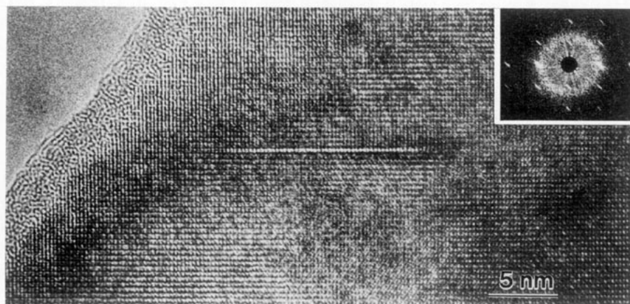
FIG. 9. \langle 110 \rangle HREM image of the TEM specimen edge with one defect close to the edge. The defect exhibits characteristic bright dumbbells. The inserted optical diffraction pattern was obtained from the amorphous specimen edge and indicates a defocus \Delta f = -40 \pm 5 nm.
